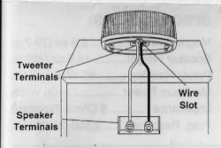
Using speaker wire (not supplied), connect the tweeter's positive (+) and negative (-) screw terminals to the corresponding terminals on your existing speaker system. Then press the wires into the slot on the bottom of the tweeter's cabinet.
