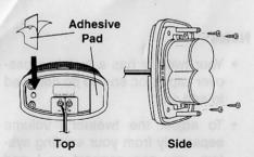
To mount the tweeter on top of an existing speaker system, peel the backing off each side of the supplied adhesive pads and press a pad onto each end of the frame on the bottom of the tweeter. Then press the base of the tweeter firmly against the mounting surface so the pads stick to the mounting surface.
