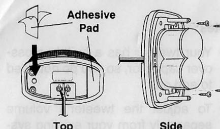
*To mount the tweeter on top of an existing speaker system, peel the backing off each side of the supplied adhesive pads and press a pad onto each end of the frame on the bottom of the tweeter. Then press the base of the tweeter firmly against the mounting surface so the pads stick to the mounting surface.*
