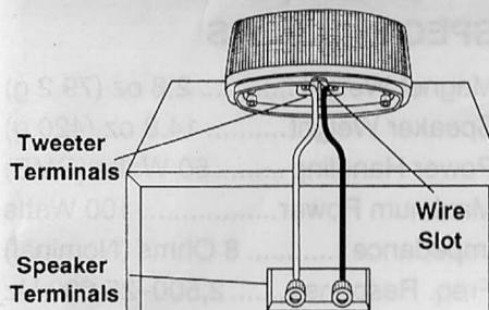
Using speaker wire (not supplied), connect the tweeter's positive (+) and negative (-) screw terminals to the corresponding terminals on your existing speaker system. Then press the wires into the slot on the bottom of the tweeter's cabinet.
